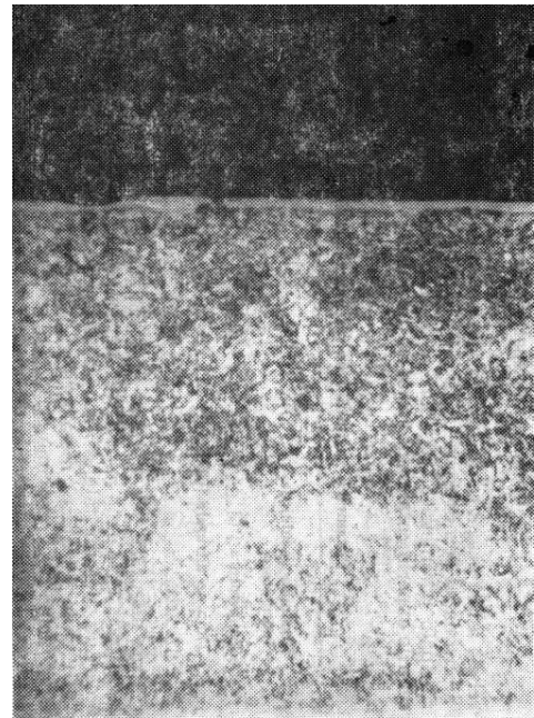
Figure 8. Microstructure (x 500) in the cross-section of a plasma nitrided test sample made of 40Cr4 (hardened initial state) 12h / 550°C
